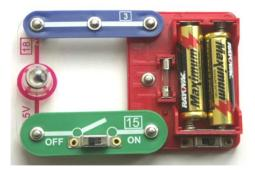
Slide the switch 15 to the ON position, the bulb should light up. If it does not, first check that the bulb is screwed properly into the bulb holder and if this does not work, try some fresh batteries.
