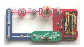
It is called a series circuit because the electricity has to go through each of the components before it can get back into the battery so in this circuit, the motor and the lamp share the 3 Volts.
